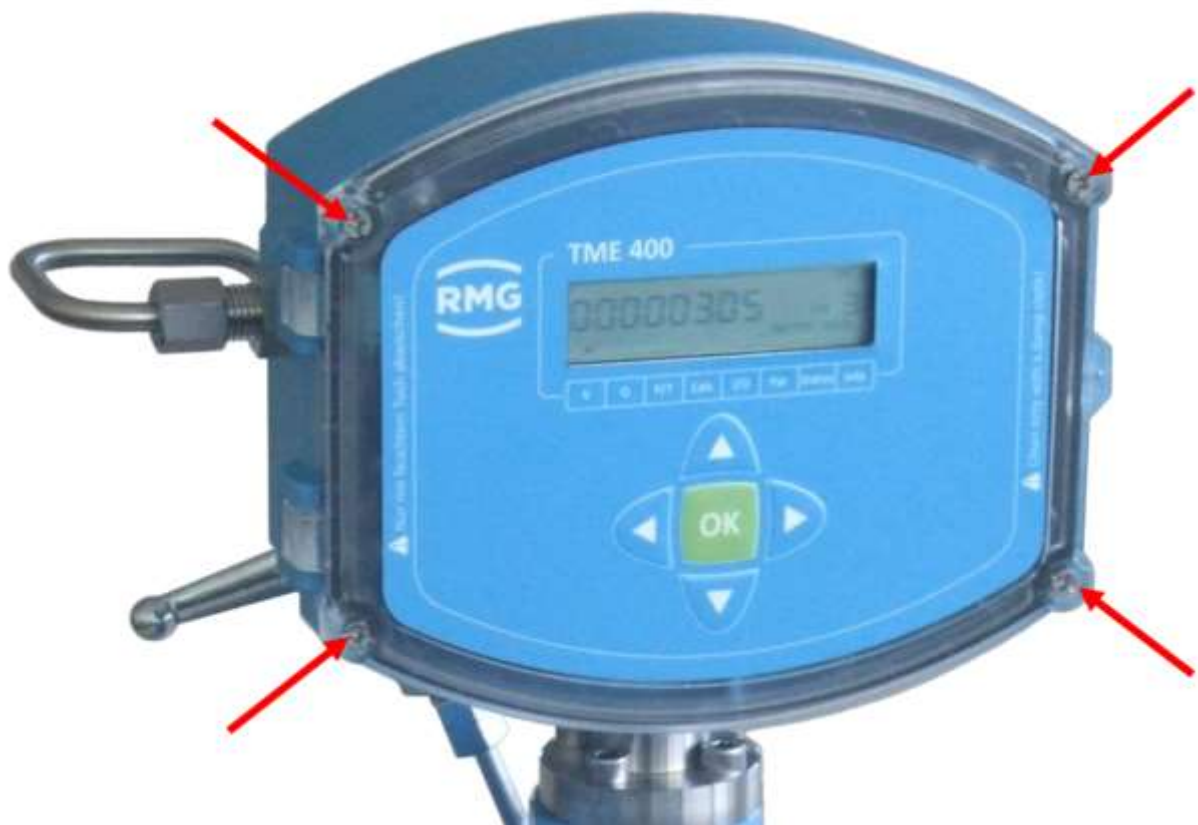
Figure 3: Unscrewing the screws to open the cover
