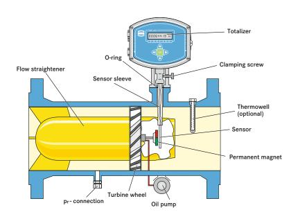
Furthermore, the volume corrector integrated in the TME 400-VCF allows the calculation of the standard volume (VB). In order to do this, the meter measures operating pressure and operating temperature in addition to the operating volume flow. From this, the standard volume flow can be calculated using a suitable equation of state together with the corresponding standard conditions. Then this value is summed up in the standard volume totalizer and stored in the data logger.
