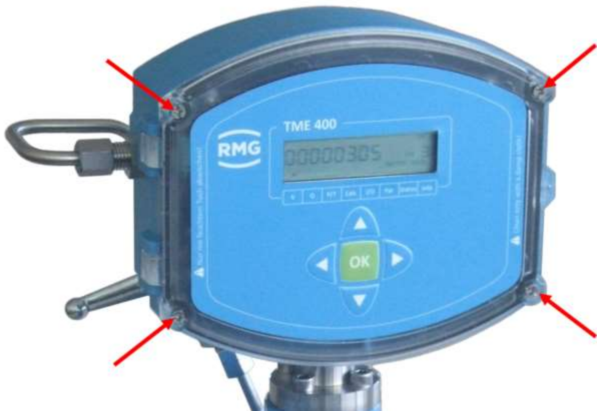
Figure 3: Unscrewing the screws to open the cover
