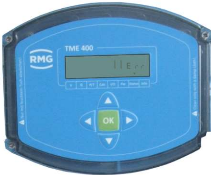
Figure 18: Error message in the display
