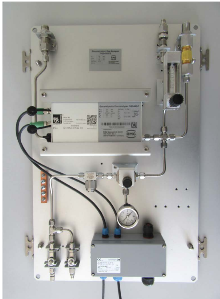
Figure 2: Photo GQS 400-FS with fine pressure reduction
