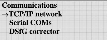
The arrow is located on the second line and can be moved upwards or downwards using the cursor keys. In this example, you have to use the **Cursor Down** key until DSfG corrector appears. Then press **Enter** to select the **DSfG corrector** chapter. A new window will open with the **DSfG corrector** heading. The contents of this chapter can be browsed using the cursor keys.
