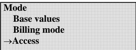
The arrow is already located on the third line on Access. In this example, pressing **Enter** will select the correct chapter. A new window will open with the **Access** heading. Use the **Cursor Down** key to select the first codeword.
