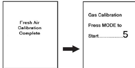
Press the Mode button during this countdown to begin the span calibration. The monitor will display a prompt for the appropriate calibration gas to be applied (using the adaptor as illustrated below).
