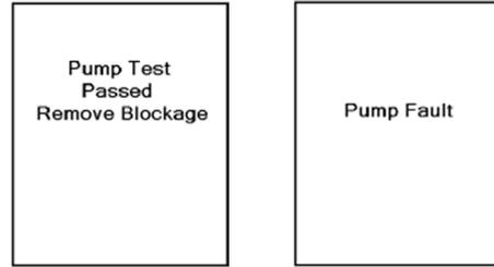
If a monitor fails the pump test, remove it from service until the fault is found and corrected. The most common cause for failure is having one of the two internal filters plugged. This fault is field-serviceable. (See section 6.5.1 of the reference manual.)
