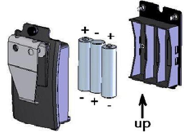
Reattach the cover plate and reinsert the battery pack back in the monitor.
