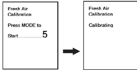
Press the Mode button again during this countdown to begin the zero calibration.
