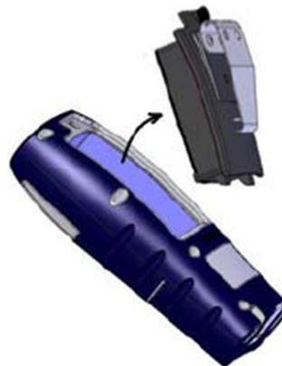
To replace alkaline batteries, remove the cover plate on the battery pack by rotating the two screws a quarter-turn counterclockwise. Pull out the old batteries and replace them with new batteries in the same orientation (see illustration).
