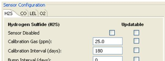
**Figure 7. Sensor Configuration Tab (H<sub>2</sub>S) via MicroDock II**
