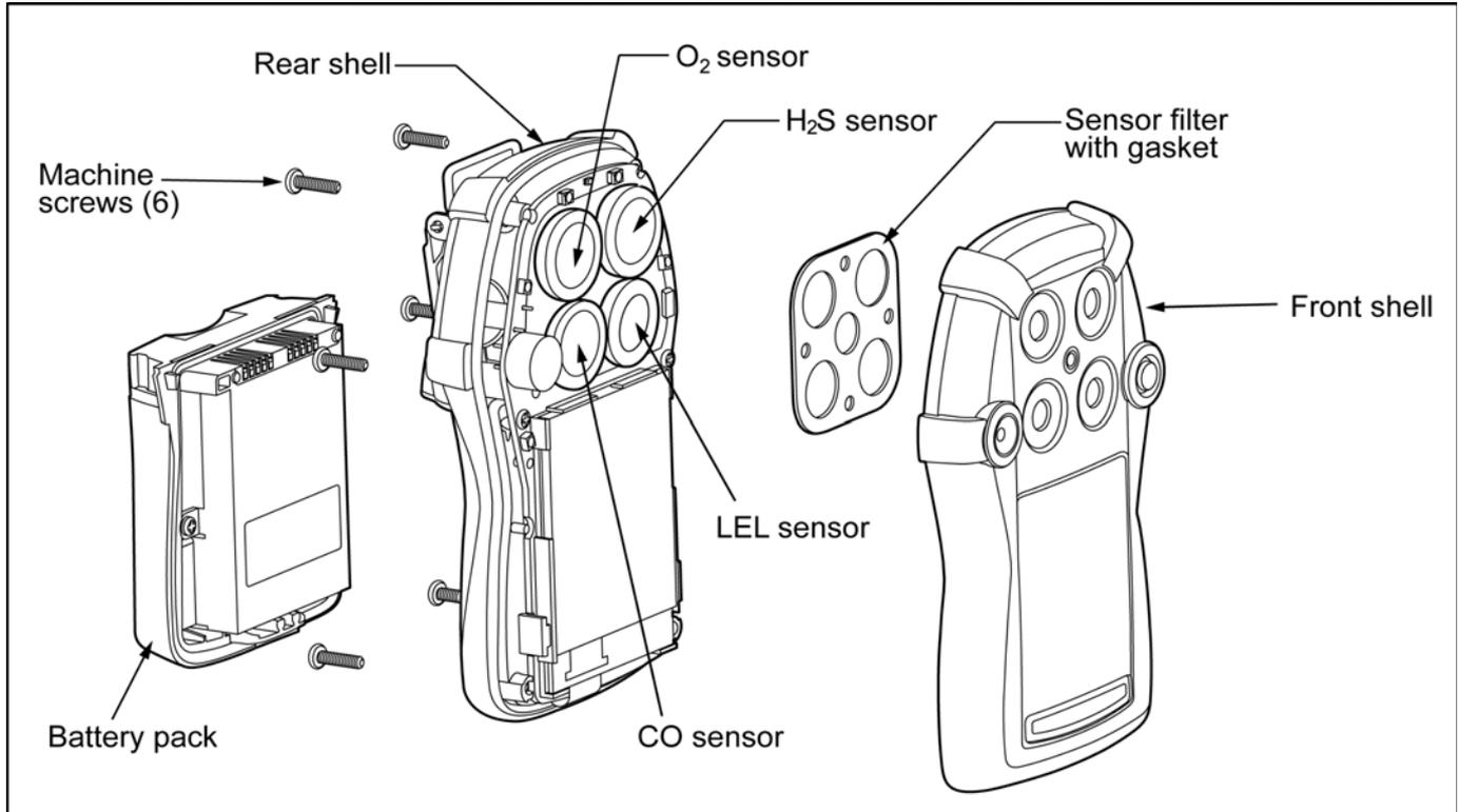
**Figure 23. Replacing a Sensor or Sensor Filter**
