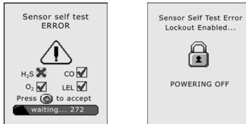
**OFF** then displays and the detector deactivates. For all sensor and self-test error screens, refer to [Startup Troubleshooting](#).
