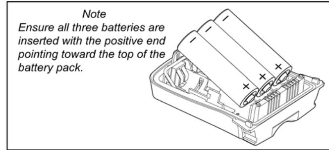
**Figure 22. Inserting the Alkaline Batteries**
