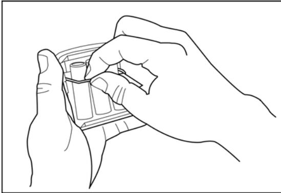
**Figure 21. Pulling up on the Ejector Bar**
