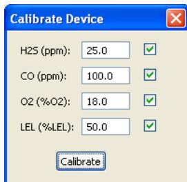
**Figure 15. Calibrate Device Dialog Box**
