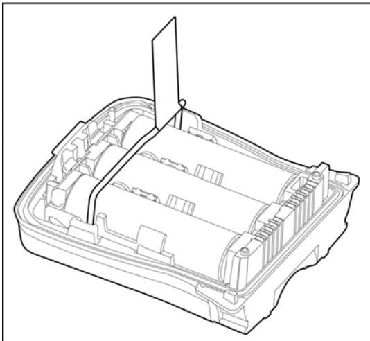
**Figure 19. Ejector Bar Unhooked from Release Clasp**
