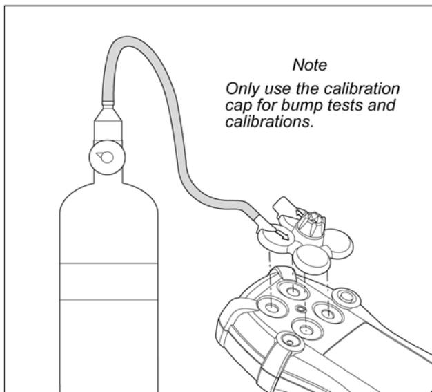
**Figure 11. Connecting the Gas Cylinder to the Detector**
