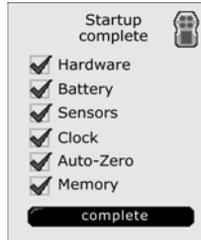
If ✘ displays for Hardware, Battery, Sensors, Clock, or Memory contact [BW Technologies by Honeywell](#). If an ✘ displays Auto-Zero, the detector uses the previous zero readings. The detector can be zeroed in a safe area free of hazardous gas. Refer to steps #1-9 in [Quad Gas Calibration](#).
