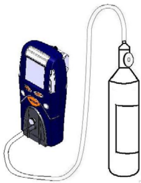
Figure 4.1 Bump Test / Gas calibration set up
